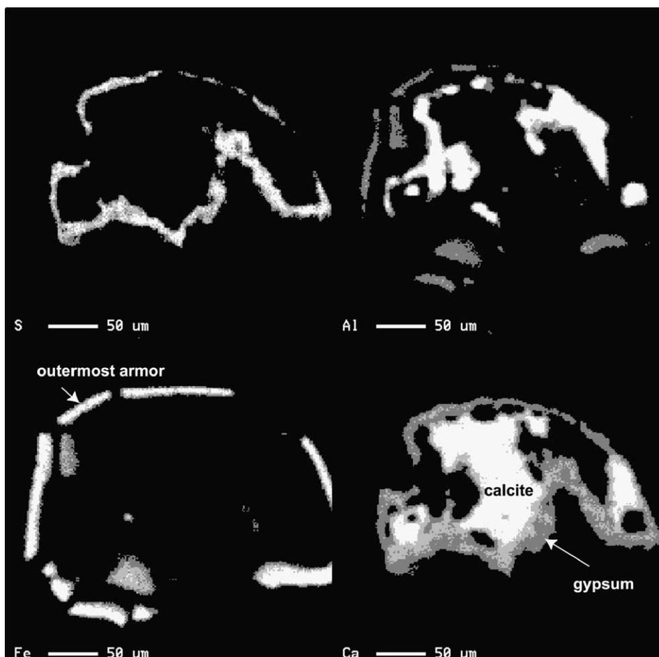
Fig. 8. Map of element distributions across a partially dissolved, armored limestone grain after 48 h of exposure to Friendship Hill AMD. White represents the highest concentration of the element in the field of view. The calcite core is deeply embayed and surrounded by a layer of gypsum (Ca and S). An Al-rich zone forms between the gypsum and the outermost Fe armor.
