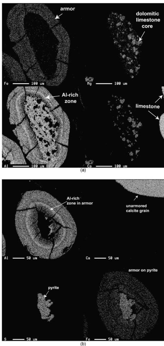
Fig. 10. Maps showing the distribution of elements in refractory grains in reactor limestone: (a) zoned Fe- and Al-rich 50- $\mu\text{m}$  thick armor coating developed on dolomitic limestone. Adjacent calcite-rich limestone grains (see Ca map) are rounded, but show no armor overgrowth. (b) Armored pyrite grain. Note unarmored calcite grain in upper corner of Ca map and lack of any Ca in the area of the armored pyrite grain.
