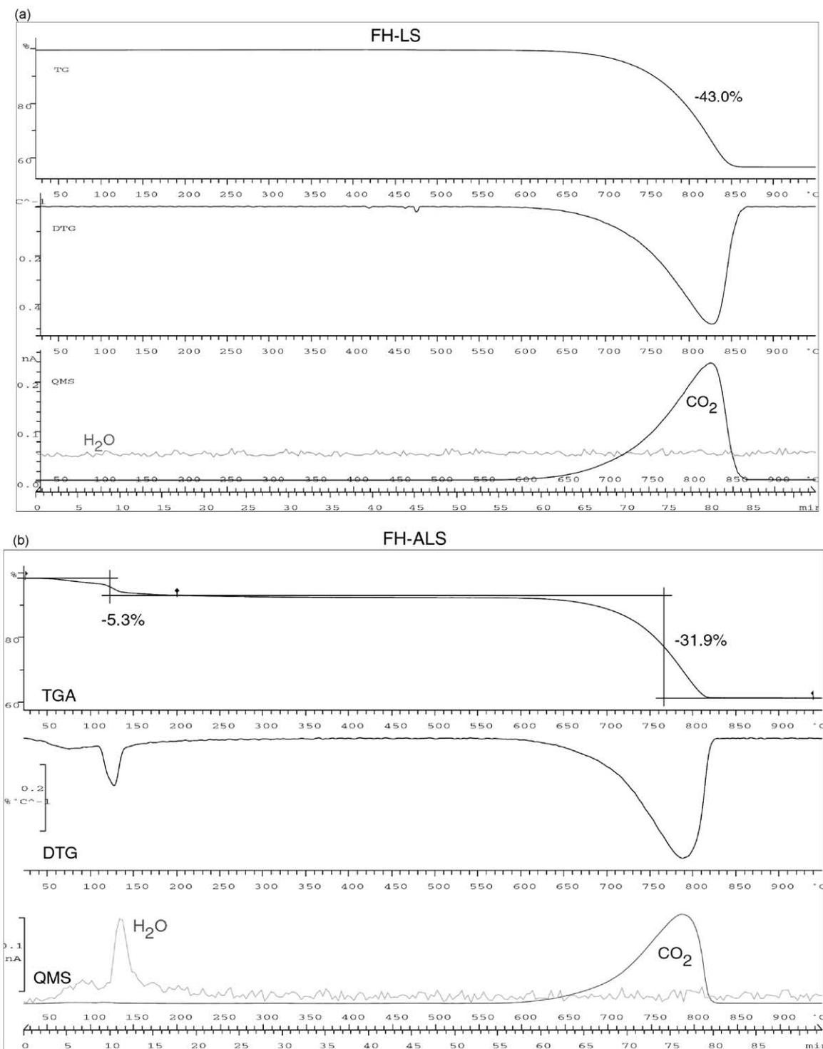
Fig. 3. Thermogravimetric analysis. TGA, mass loss on heating as a function of temperature. DTG, First derivative of mass loss curve. QMS, Quadrupole mass spectrometer data for masses 18 (H<sub>2</sub>O) and 44 (CO<sub>2</sub>). Samples were heated from 22 to 950 °C at a rate of 10 °C/min in an Ar atmosphere. (a) Limestone feed material sample FH-LS (23.5 mg starting sample mass); (b) armored limestone sample FH-ALS (15.8 mg starting sample mass).
