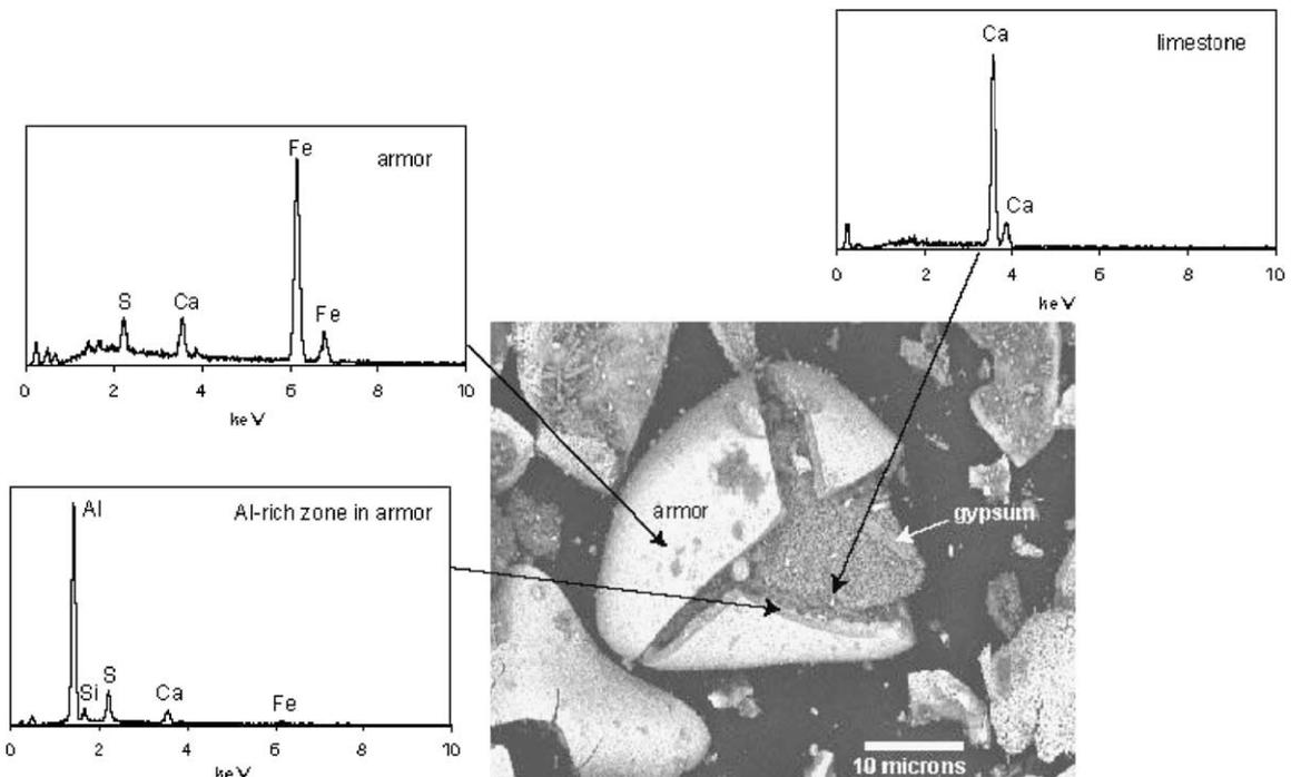
Fig. 6. EDS spectra for armored limestone. The interior of the armor shell is Al-rich relative to the Fe- and S-rich outermost material.
