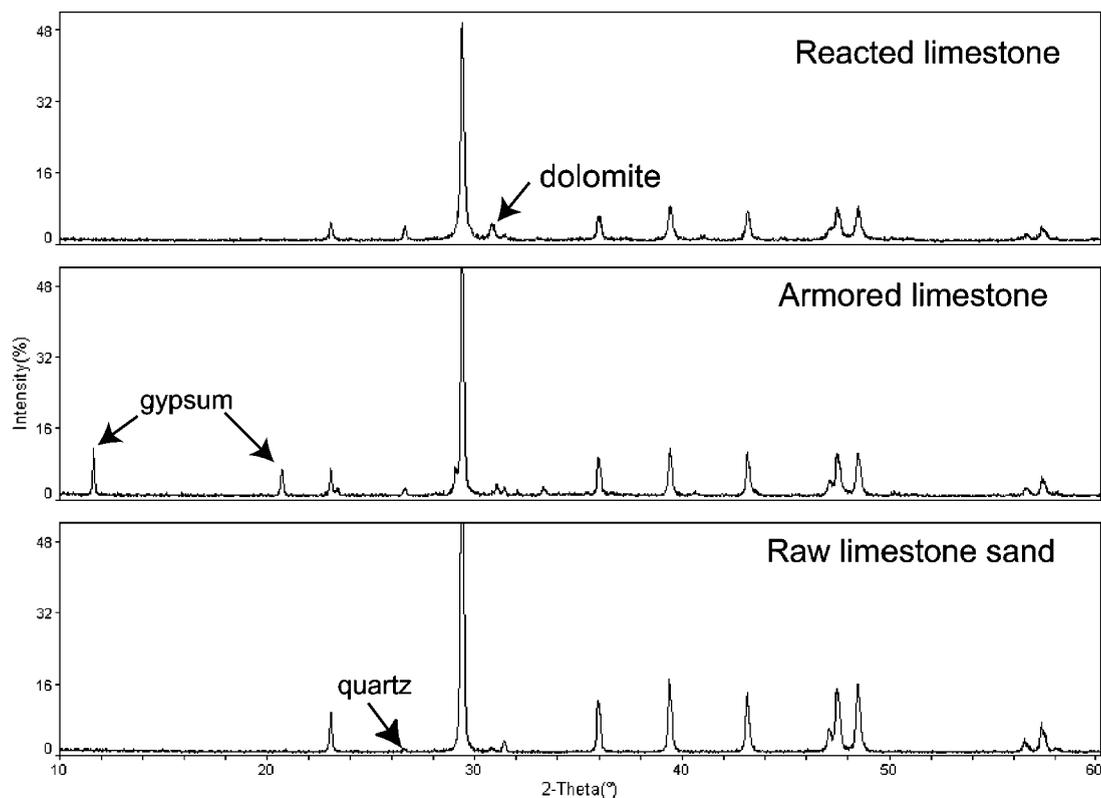
Fig. 2. X-ray powder diffraction patterns for raw limestone sand, armored limestone and reactor limestone. All unlabelled peaks match calcite, quartz, and dolomite.
