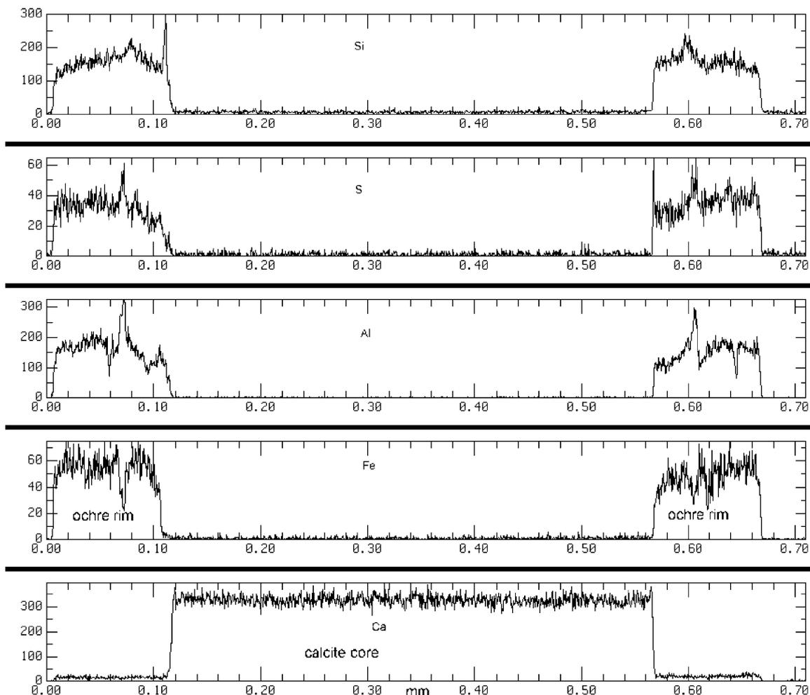
Fig. 9. Traverse across an armored calcite grain in the reactor limestone. Plots show counts as a function of distance. Note the absence of gypsum and the spikes in Al and S concentrations at a distance of 0.07 mm into the grain and again at 0.61 mm on the opposite side of the calcite core.
