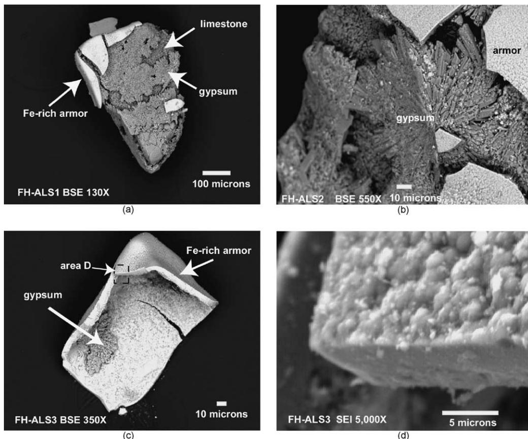
Fig. 5. SEM images of armored limestone: (a) partly armored grain showing gypsum coating on limestone surface; (b) close-up view showing well-developed sprays of gypsum crystals; (c) armor coating broken off limestone core. Note patch of gypsum adhering to inner armor lining. (d) High magnification image of outer armor showing rounded, colloidal-size particles.
