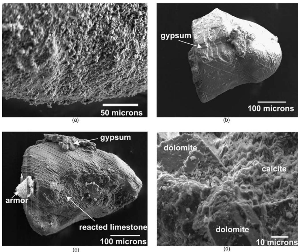
Fig. 4. SEM secondary-electron images of limestone surfaces: (a) raw limestone sand; (b) well-developed gypsum coating on a rounded limestone grain from the 48-h armoring experiment. Armor coating removed by sieving. (c) Reactor limestone grain with a patch of gypsum and armor coating. Note the striations and surface relief developed on the rounded limestone grain. (d) Refractory dolomite (smooth) and etched calcite in reactor limestone.
