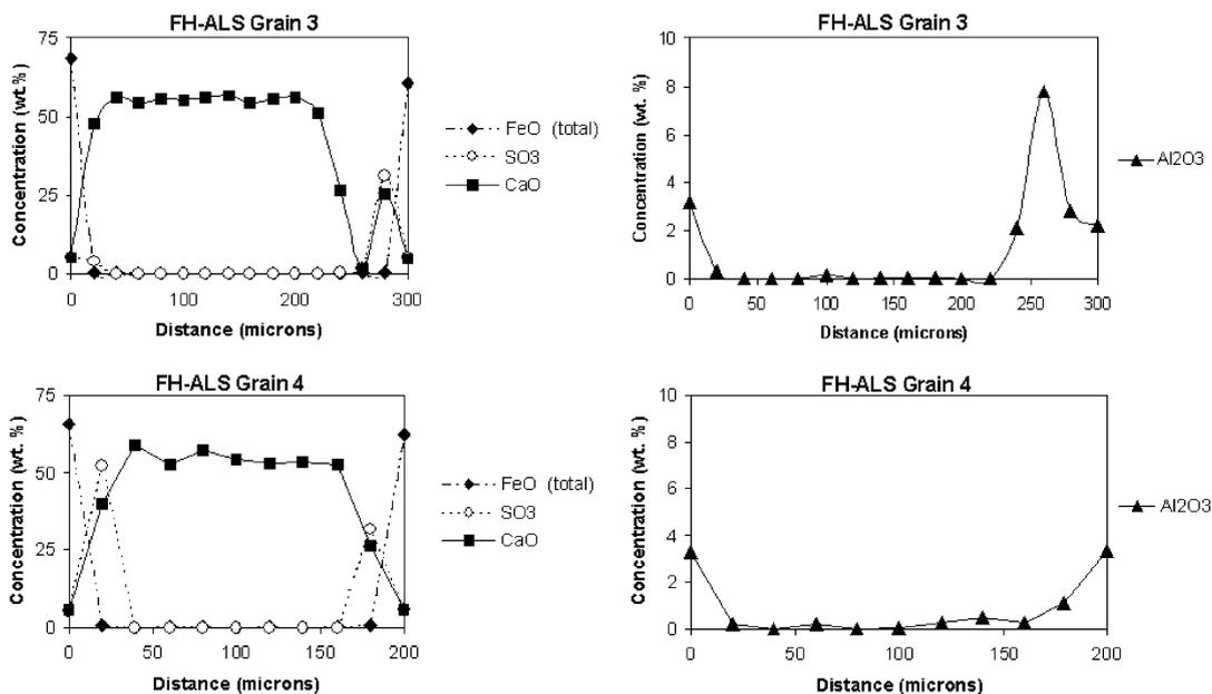
Fig. 7. Electron microprobe point analysis traverses across two armored limestone grains. Traverses start on the Fe-rich armored rim and step across the grain in 20- $\mu\text{m}$  increments, passing through the unaltered limestone core. Note the gypsum rind (elevated CaO and  $\text{SO}_3$ ) at the edge of the limestone core. Alumina increases at the edge of the grains.
